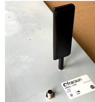
Figure 8-1: Blade antenna oriented straight and connected to SMA connector
