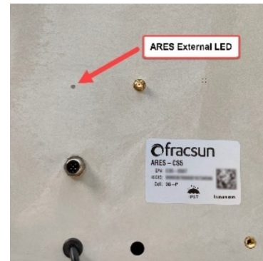
Figure 9-1: ARES external LED location
