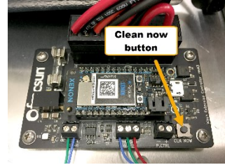
Figure 10-9: Manually test the pump with this button
