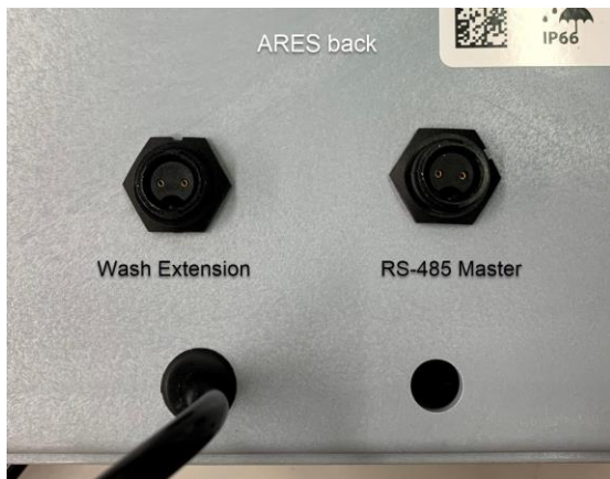
Figure 3: ARES additional RS-485 connection (factory)
