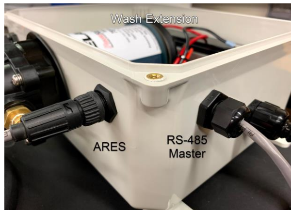
Figure 4: Wash Extension additional RS-485 connection
